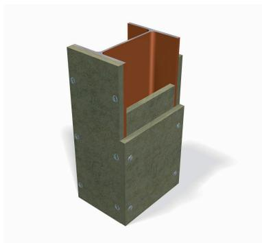
**2** Press the pieces of insulation between the flanges behind a coming joint.
